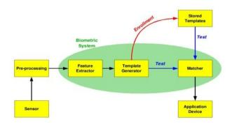
Figure 2: Basic structure of biometric authentication system
